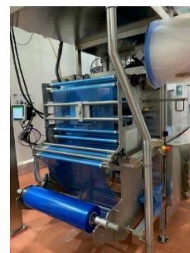
Figure 4- OPA/PE film prior to grated cheese being processed and packed. Blue packaging is mandatory in food manufacturing.
